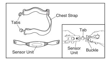
Next, wrap the chest pulse sensor around your chest and attach the other end of the chest strap to the sensor unit. Adjust the length of the chest strap, if necessary. The chest pulse
